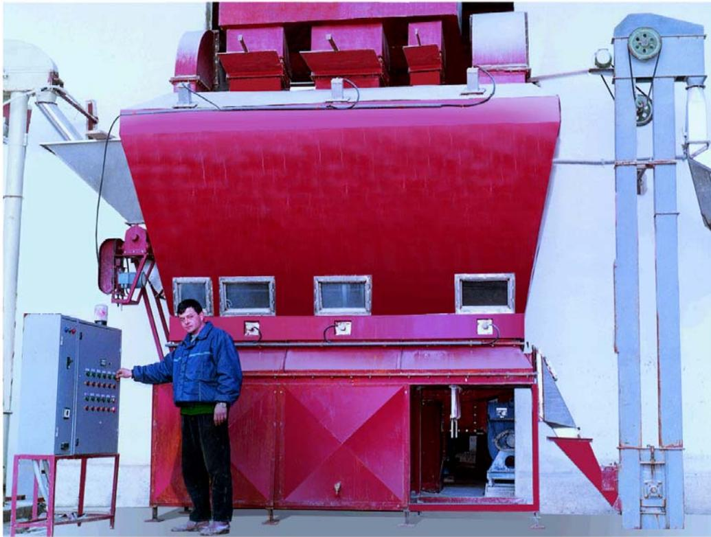
Figure 1. Rotation-pulsed fluid bed working chamber.
